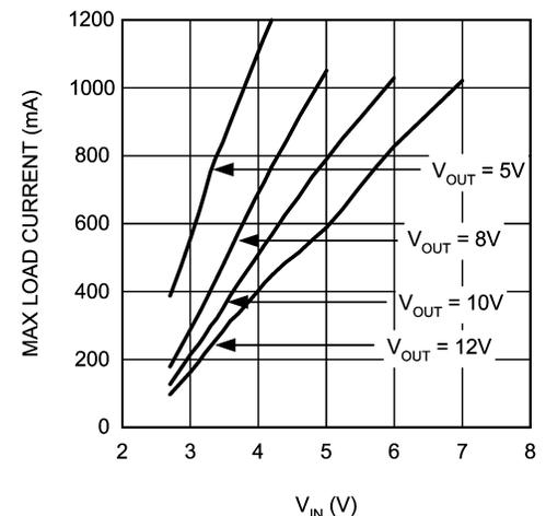
Max. Load Current (typ) vs  $V_{\text{IN}}$  - "Y"
