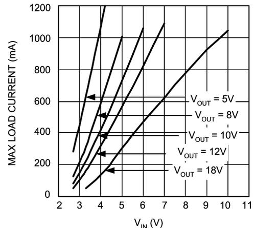
Max. Load Current (typ) vs  $V_{\text{IN}}$  - "X"
